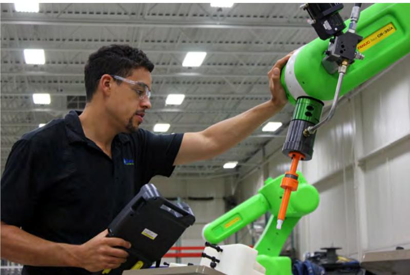
*Collaborative robot system for dispensing urethane to automotive glass.*
